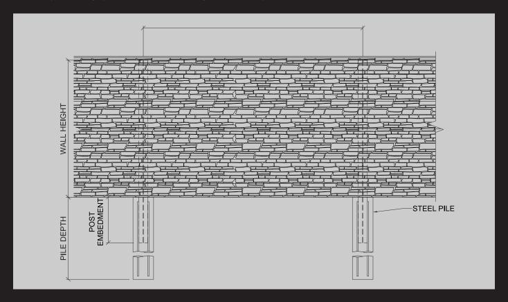
**StoneCrete** walls are available in standard heights of 300mm - 1800mm (1ft - 6ft) with standard lengths of 4.8m between post columns. Our wall system may be engineered to be stacked in order to accommodate higher heights if desired.
