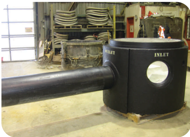
HDPE cast into barrel - watertight.
