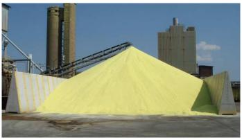
Requiring only a structurally solid base to sit on, the precast concrete wall units can be used in a variety of applications. Units come in six sizes from 1.2m to 6.0m and can weigh up to 5.2 tonnes. The Alfabloc® has been tried and tested over many years of constant use and can withstand significant impact by mechanical plant as well as withstanding extreme weather conditions. Alfablocs® are used in many sectors including Agriculture, Waste & Recycling, Ports & Shipping etc.
